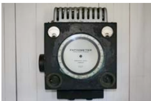
Figure 2 Reginald Aubrey Fessenden 100 Fathometer – Sonar (iceberg and water depth sounder).
